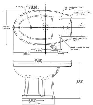
Hydraulic performance, water surface area, trap seal depth, and all fixture dimensions meet or exceed ASME Standard A112.19.2 requirements.
